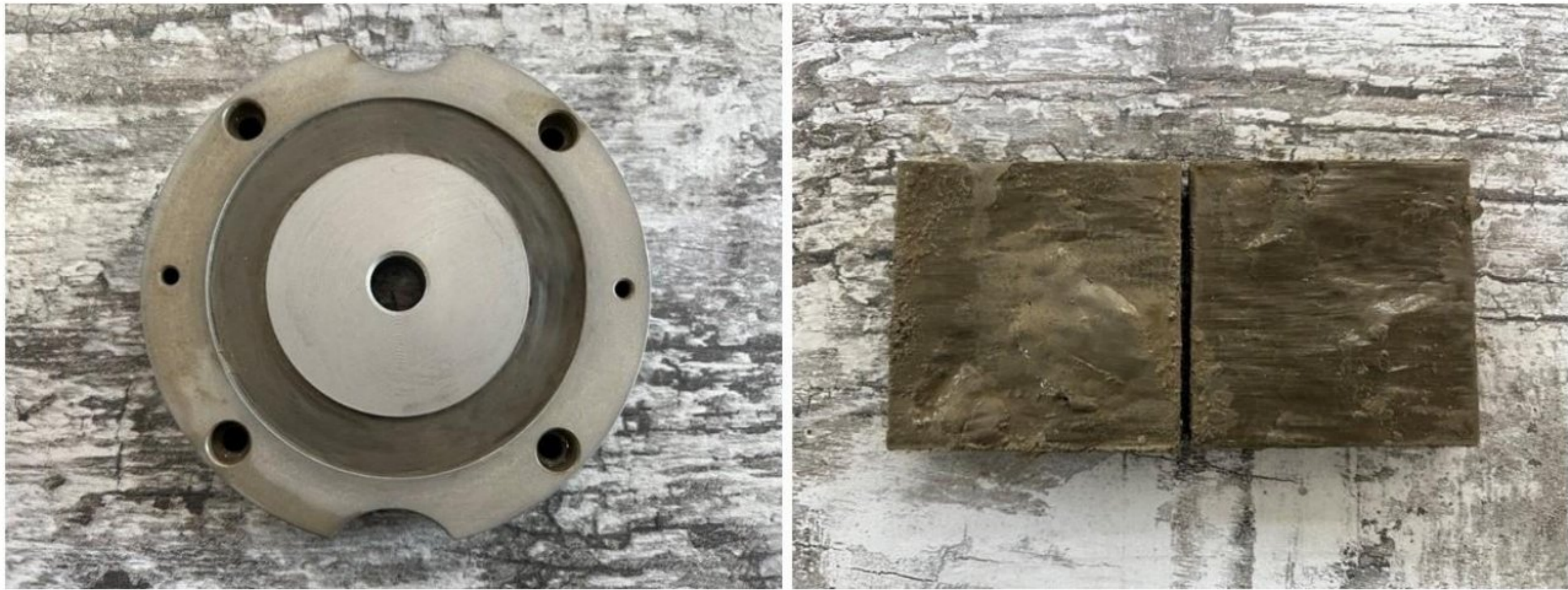
Figure 5. Appearance of the gray clay samples after testing in the ring shear apparatus ( left ) and direct shear apparatus ( right ).
