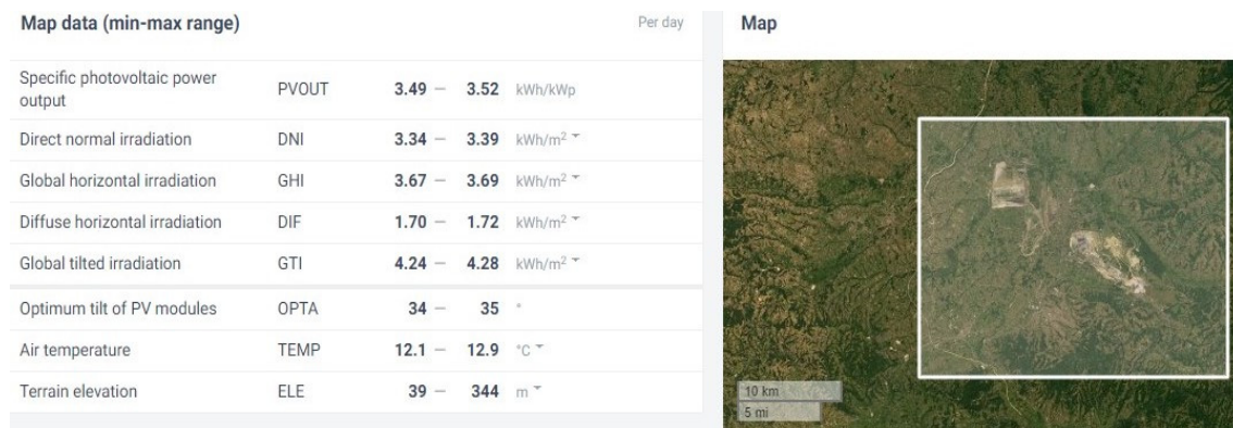
Figure 4. Coal basin Kolubara west (available flat surface 1900 ha) and east opencast mine area photovoltaic possibilities (available flat surface 1700 ha) (data obtained from the “Global Solar Atlas 2.0, a free, web-based application is developed and operated by the company Solargis s.r.o. on behalf of the World Bank Group, utilizing Solargis data, with funding provided by the Energy Sector Management Assistance Program (ESMAP). For additional information: https://globalsolaratlas.info ) [9].
