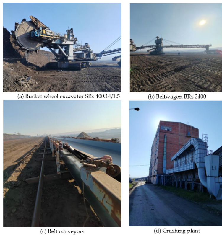
Figure 2. I ECC system at the open pit Drmno with parts of system—(a) Bucket wheel excavator, (b) Beltwagon BRs 2400, (c) Belt conveyors, (d) Crushing plant (photographed by M.G.).
