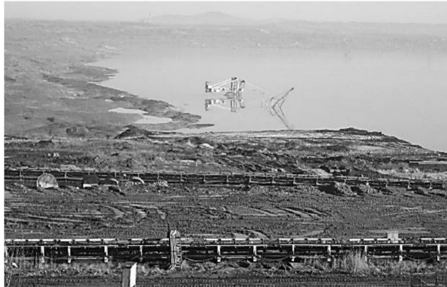
Figure 4, Submerged working slopes, dumper and spilled sand rampart in the foreground part of the internal landfill of OP "Tamnava-West field" during pumping out (13/01/2015)
